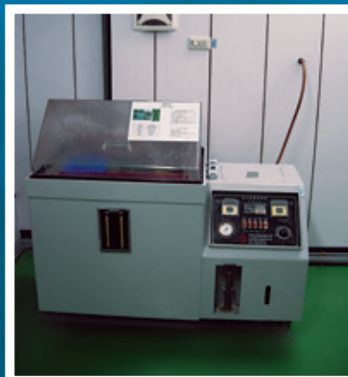
6. 鹽水噴霧測試機台 Salt spray tester
