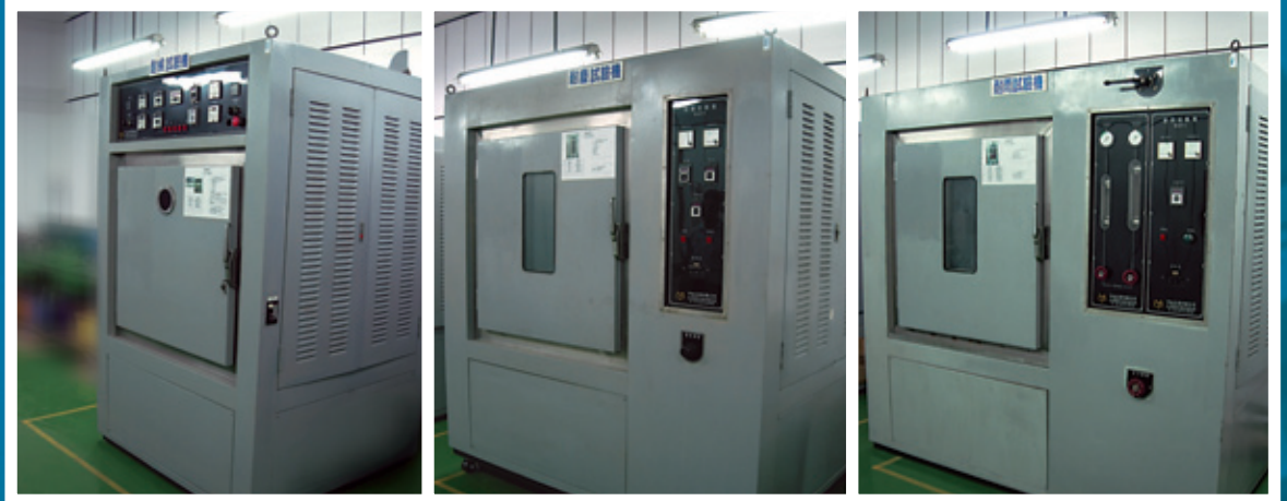
1. 耐候測試機台 Weather meter
